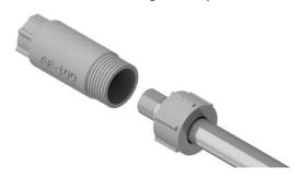
c) Reattach the cap to the expansion fitting.
