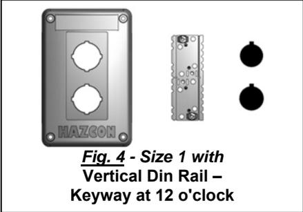
**Fig. 4 - Size 1 with Vertical Din Rail - Keyway at 12 o'clock**
