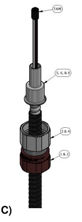
Slide the taped conductors thru the potting chamber (5) & seal (8)\* until the potting chamber rests against the armor stop. For best results, bristles should seal against the tape at the base of the cable. Ensure there are no gaps between the seal & conductors. If any gaps, use packing fiber to fill.
