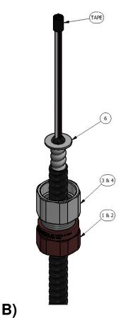
Push the prepared cable through the back nut (1), middle nut (3), and grounding spring (4). Locate the armor stop (6) at the end of the armor as shown above. If the conductors are too large to fit through the armor stop (6) it can be removed from the assembly. The entry component (9) has a builtin armor stop for larger cables.
