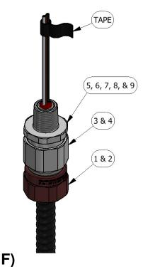
Thread the back nut (1) onto the middle nut (3) to the torque show in Table 2. This will compress the seal (2) inside the back nut (1) to grip the jacket of the cable for mechanical retention and the formation of an environmental seal. Allow the compound to fully cure before energizing the circuit.
