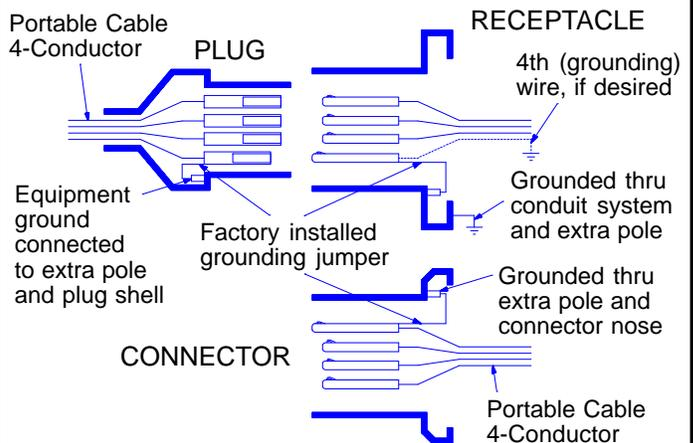
**Style 2 Plug** - Equipment grounding conductor is wired to the extra grounding contact with attached ground strap which provides a parallel ground circuit thru the extra ground pole and plug shroud. The ground stand-off and shroud are grounded to a copper alloy ground jumper installed on the extra ground pole. This, in turn, grounds the entire plug assembly housing.
