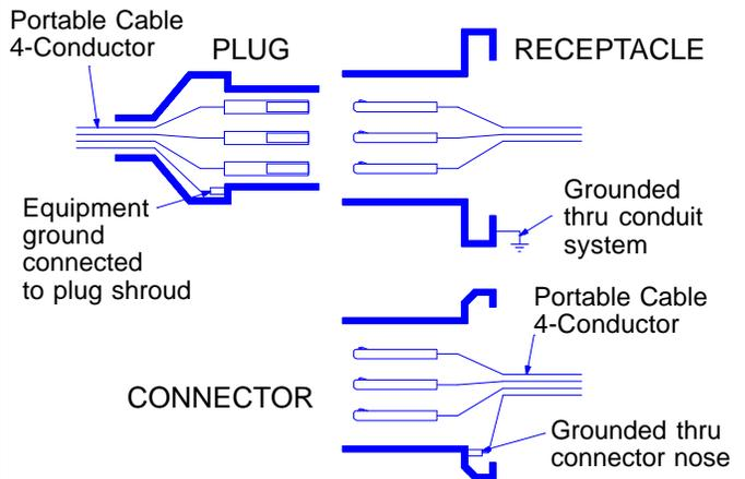
**Style 1 Plug** - Equipment grounding conductor is wired directly to the ground terminal which is connected to the ground stand-off and shroud. This, in turn, grounds the entire plug assembly housing. All contacts are "current carrying".
