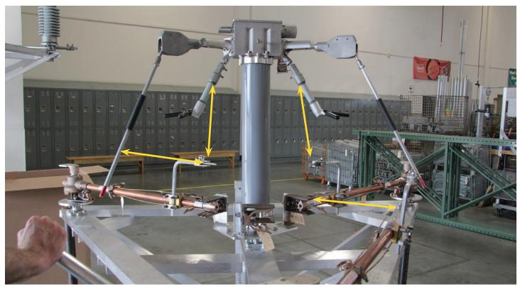
Figure 12: The "**Air Gap**" dimension listed on the setup drawing is the minimum distance allowable from metal to metal when the interrupter opens. In order for the TECORupter to operate correctly, the distances pointed out in the picture above must be greater than the air gap dimension listed on the setup drawing. Both the "pull side" and the "lag side" should be checked.
