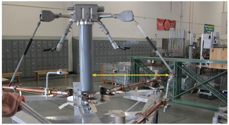
Figure 11: The "**Drops Off At**" dimension is measured from the base to the actuating rod tip at the point where the actuating rod drops off of the pick up finger. An example of the measurement is shown above.
