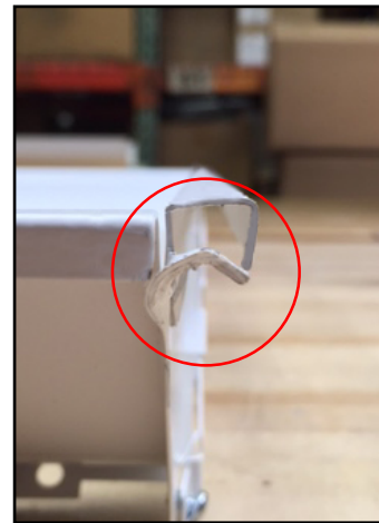
Figure 3. Hinge Front View (Incorrectly Aligned)
