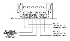
CAUTION: The sum of loads connected to Output Circuits 1 and 2 must not exceed unit rating in emergency mode.
