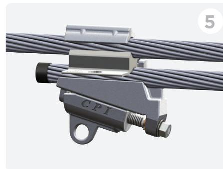
Installation is now complete. To remove the connector, use a 9/16 socket to unscrew the bolt completely and remove the assembly.
