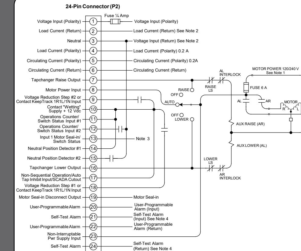
**⚠ WARNING:** When an adapter panel is not used, automatic shorting of CT inputs is not provided by the M2001D/M-2050; the customer must provide a method for shorting the CT's before the control is disconnected.
