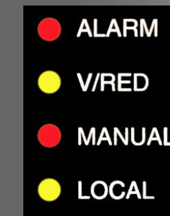
**ALARM LED** Indicates any of the programmable alarms are activated.
