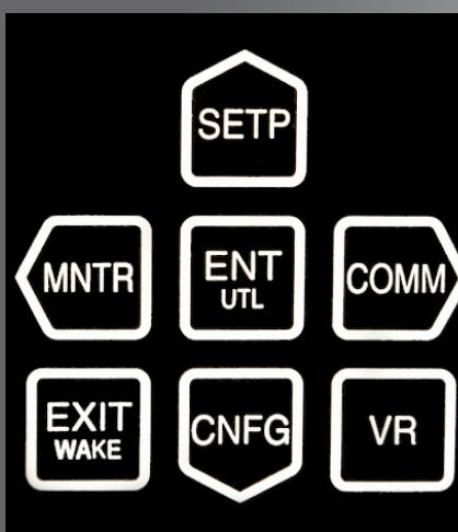
**EXIT/WAKE Pushbutton** The EXIT WAKE Pushbutton wakes the LCD from sleep mode and begins scrolling through a list of user programmed metered/calculated values.
