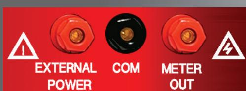
**CAUTION:** Do not reverse the ground and hot wires when connecting an external source. A 3 AG fuse (F1) is installed to protect the control from damage if these connections are accidentally reversed. With the VOLTAGE SOURCE switch in the EXT position, the sensing and switch power circuits are connected to the external Power binding post on the front panel.
