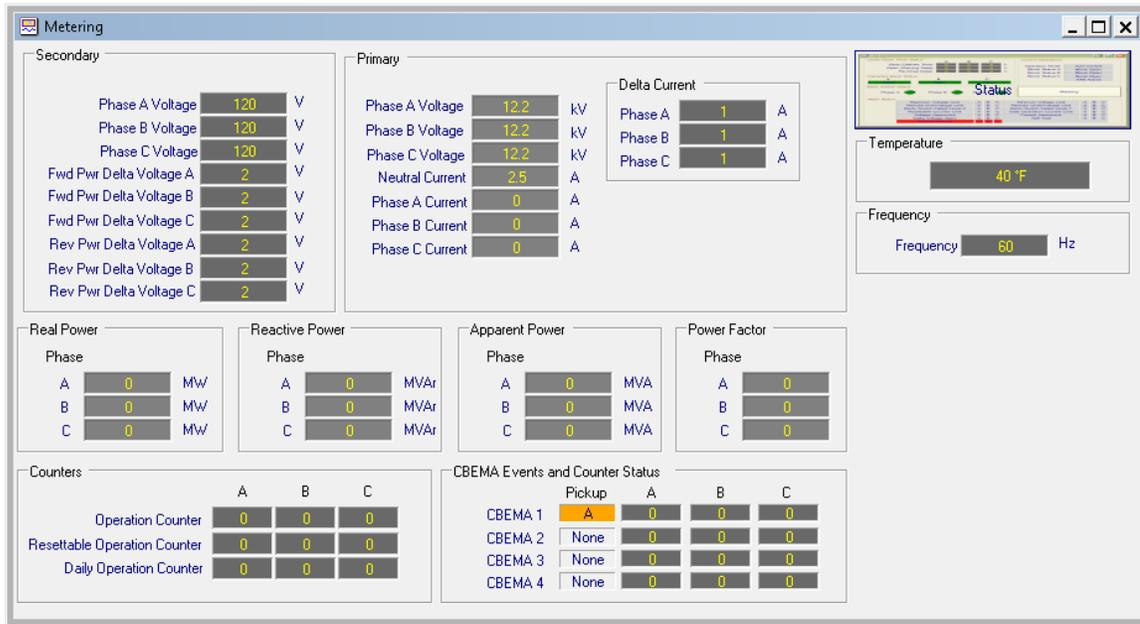
■ **NOTE:** Phase Current, Real Power, Reactive Power, Apparent Power and Power Factor are only available with the VAr Control Mode option.
