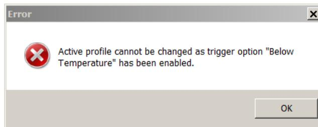
Figure 3-19 Profile Switching Warning Message Example
