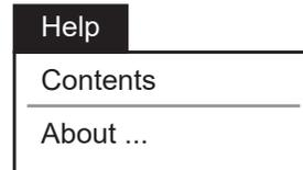
The Help toolbar item provides the user with information about the control and the software version that is installed in the unit.
