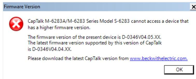
Figure 4-18 CapTalk Firmware Version Incompatibility Error Screen
