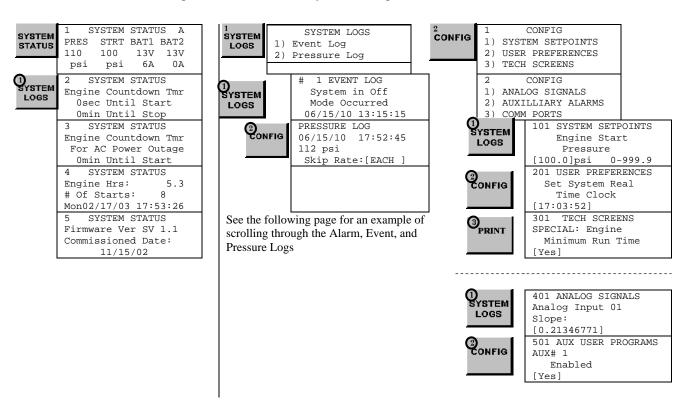
**SYSTEM LOGS:** The FD4 has three separate data logs; 1) alarm log, 2) event log, and 3) pressure log. The alarm log is a subset of the event log and only displays the last ten alarms that have occurred or cleared. The event log records all alarm and system function type events
