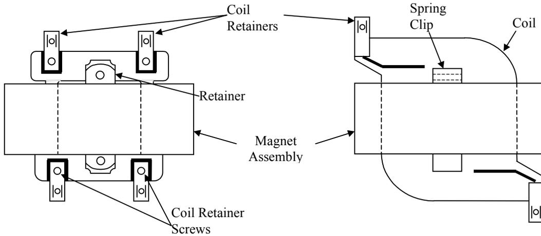
**Figure VI-1 Magnet Assembly and Retainers**
