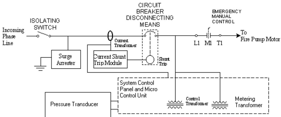
Figure 1 **Block diagram of Across-The-Line type Controller showing one phase**
