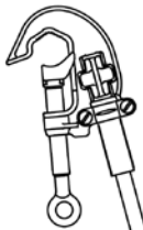
Pressure-type grounding-clamp uses Plain-plug type ferrules
