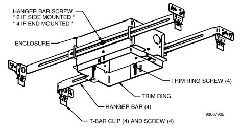
The rectangular light pattern emitted from the PECEM is oriented the same as the rectangular enclosure. Choose from below the corresponding mounting method accordingly:
