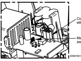
Connect both batteries to the circuit board as shown. Connect either battery to the left or right header.
