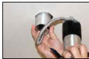
Squeeze retention springs, insert light engine assembly into the cutout, and push until springs pop out above the ceiling, locking the fixture into place. NOTE: When installing the P8153, it should be noted that the fixture will only turn in the counterclockwise direction after installation. With this in mind, point fixture lens relatively close to final desired position when inserting into ceiling. See diagram below.
