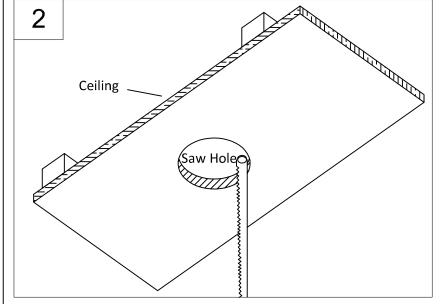
2. Use the mounting bracket as a template to create saw hole in the ceiling.
