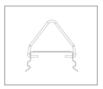
2.Secure mounting clips to housing recesses by firmly pressing them into place until both sides of the clip are secured. Hang fixture from customer supplied chain using V-brackets.
