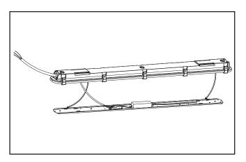
Secure mounting clips to housing recesses by firmly pressing them into place until both sides of the clip are secured.
