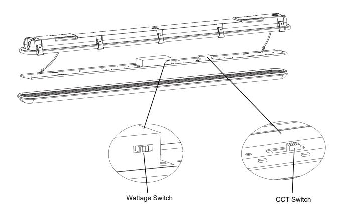
The installer may adjust the color temperature and lumen output respectively by the two DIP switch buttons integrated into the driver. Each DIP switch is accommodated with 3 options (left, middle and right), corresponding to 3 color temperatures and 3 powers respectively, which can perform the desired color temperature and lumen output combination.
