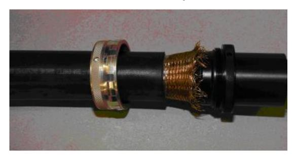
IMPORTANT: Engage the threads on the silver ring and the black ring and turn only the knurled ring on the black part to tighten. Be careful to not twist the cable braid.
