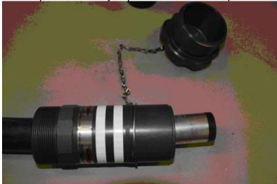
7. Slide the retaining nut onto the cable adapter.
