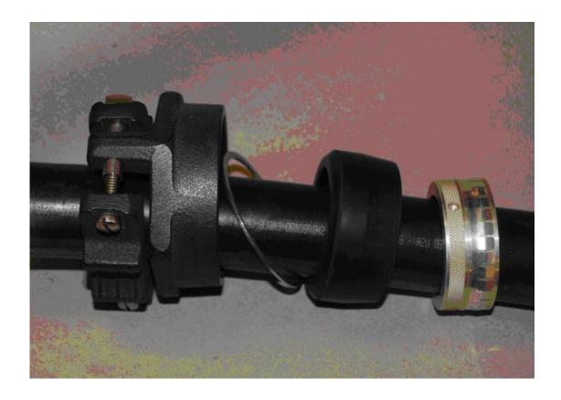
4. Slide black section of braid trap onto cable and place braid over the tapered end of the black section. Ensure that the braid is placed under the silver ring and over the lip of the black ring. Turn only the knurled ring on the black section to tighten the assembly onto the cable braid. DO NOT allow the silver ring to turn relative to the cable!!
