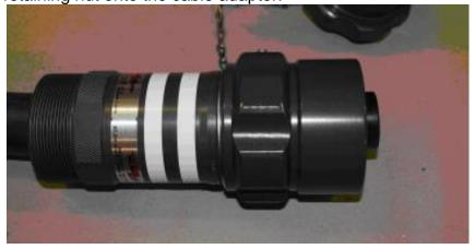
8. Install the front plug shell over the contact. NOTE: THIS ASSEMBLY IS LEFT HAND THREADED!
