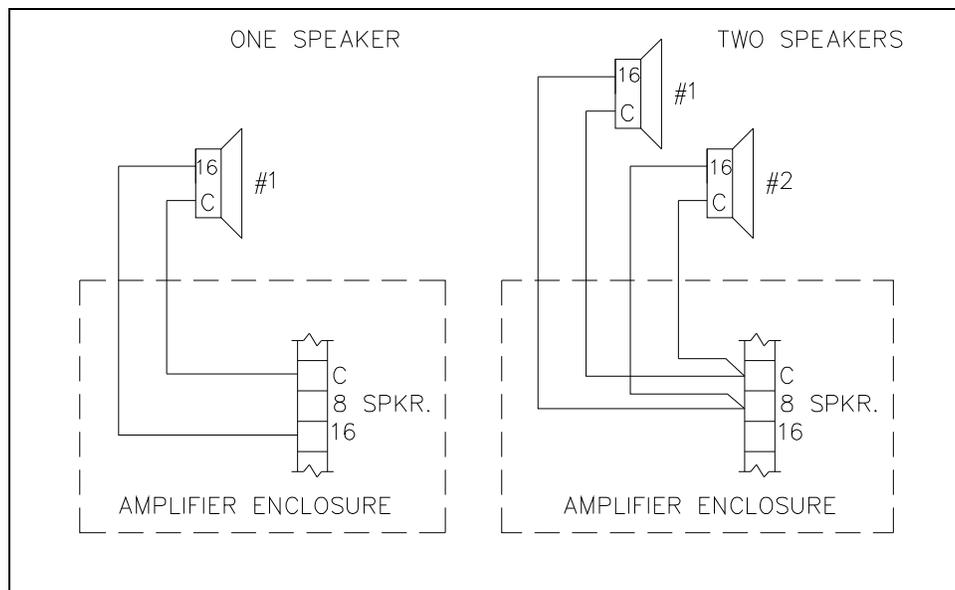
Figure 2. 16-ohm Speaker Connections
