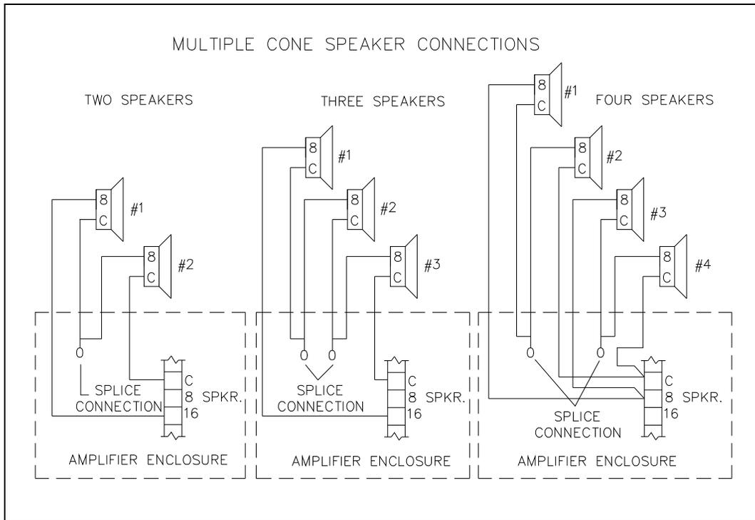
Figure 1. Cone Speaker Connections
