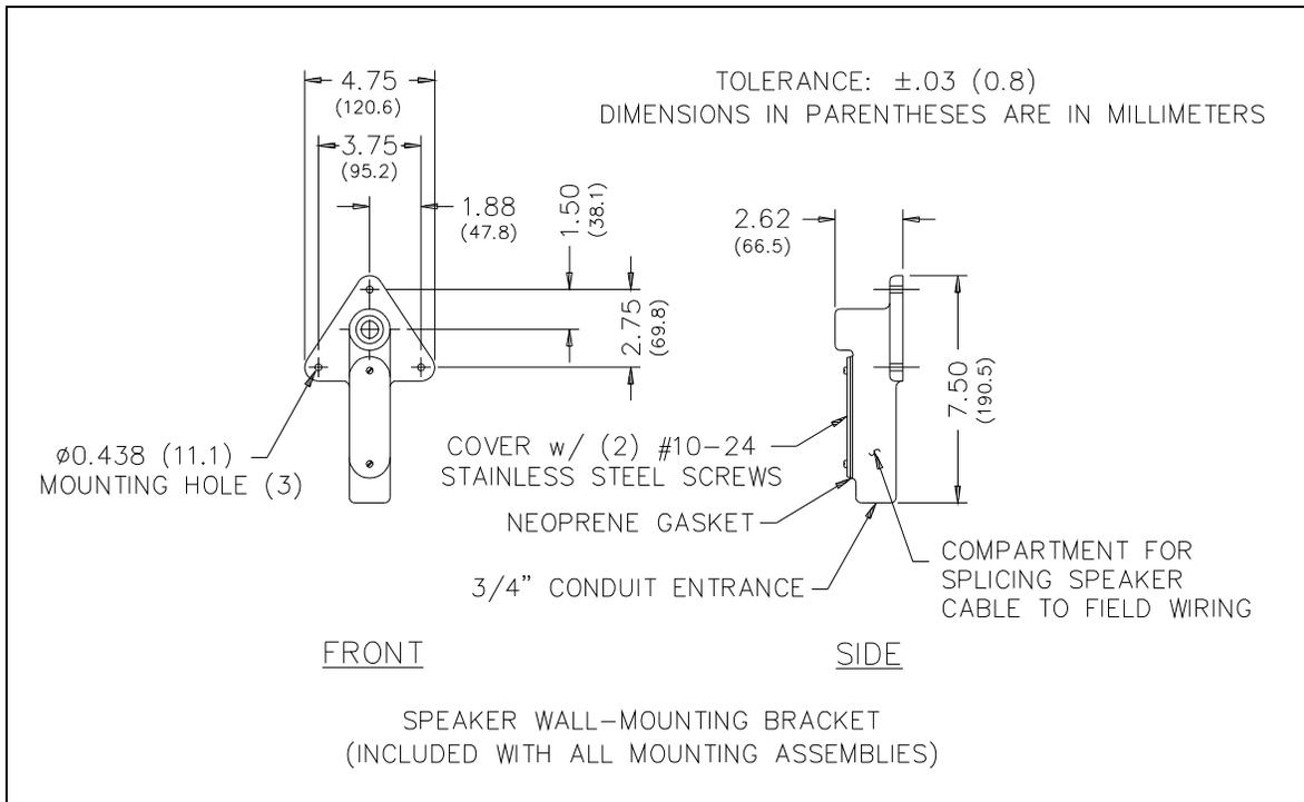
Figure 3. Wall Mounting Bracket
