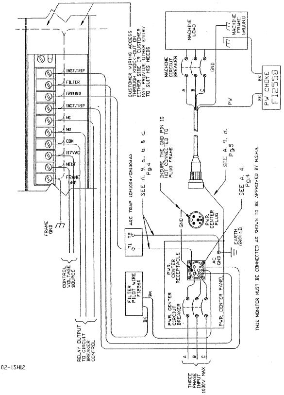
PW INSTALLATION GROUND MONITOR GM8900/40000 DO NOT CHANGE WITHOUT APPROVAL OF M.S.H.A.
