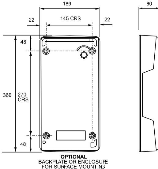
When wall or pole mounted, Sentinel telephones must be fitted inside a dedicated rear enclosure, available separately.
