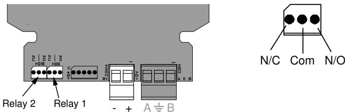
The additional outputs are provided on HD9 & HD10 as shown and are isolated SELV outputs as defined by EN 60950-1.
