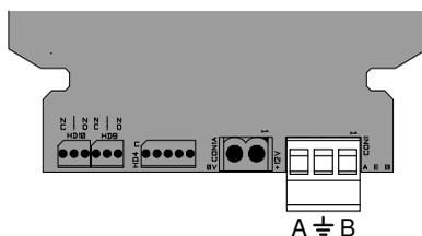
The centre earth terminal is intended for connection to a local earth to provide common mode protection from lightning transients. **If this terminal is not earthed there is an increased risk that the telephone could be damaged by line-born transients.**
