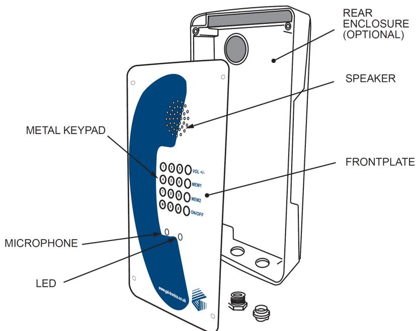
This manual describes Sentinel hands-free telephone products. These units offer high degrees of resistance to weather and abuse, having only a microphone, speaker and a rugged metal keypad mounted on a flat, metal faceplate, in place of a traditional handset. Main features include:
