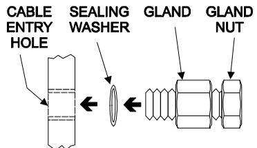
3. From the outside of the case, insert the selected gland into the threaded cable entry hole and tighten, so that its sealing washer is compressed against the enclosure surface.
