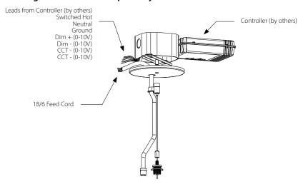
18/6 feed cord provided for wiring to pendant mounted SpectraSync luminaires. See table below for fixture to SJ cord connection recommendations.
