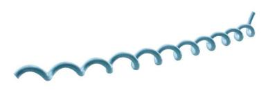
SVD's are made of material that does not abrade the cable sheath. They are designed to reduce the natural Aeolian vibration that occurs on the line by absorbing and dissipating the vibration across the damping section of the helix. The gripping section gently grips the cable to hold the damper in place without damaging the cable.
