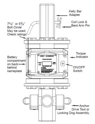
Attach Kelly bar adapter to top and anchor drive tool or locking dog assembly to bottom of torque indicator as described above. Align the Kelly bar adapter with the Kelly bar so that the cross pin holes will match up and slide the Kelly bar adapter onto the Kelly bar. Secure in place with the bent arm pin and coil lock provided with the Kelly bar adapter.
