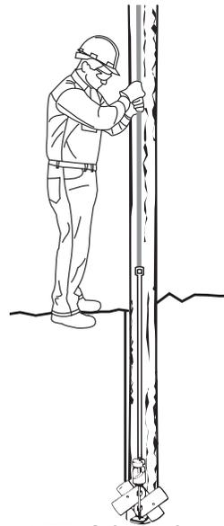
*NOTE: If desired, a second pole key anchor may be used at the top (ground level) of the hole on the opposite side*
