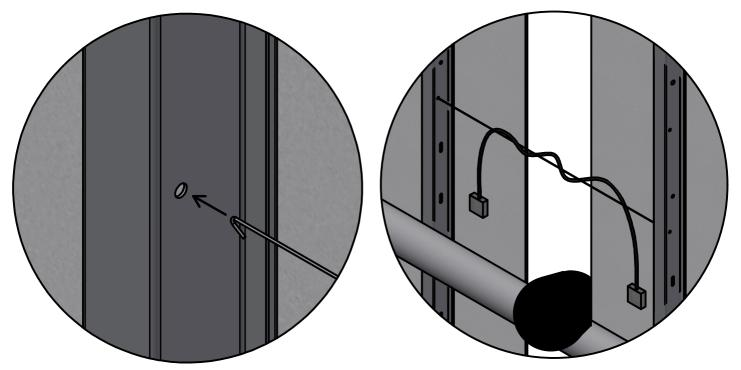
Insert one end into FS7 Wire Management hole until it snaps in place Wrap module lead around jumper 1 or 2 times, then insert opposing end into adjacent FS7 corresponding Wire Management hole
