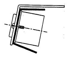
Remove and discard device mounting screws.
