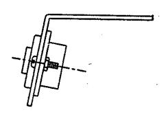
Remove and discard device mounting screws.
