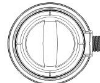
Figure 3 – Aisle lens installed 90°
