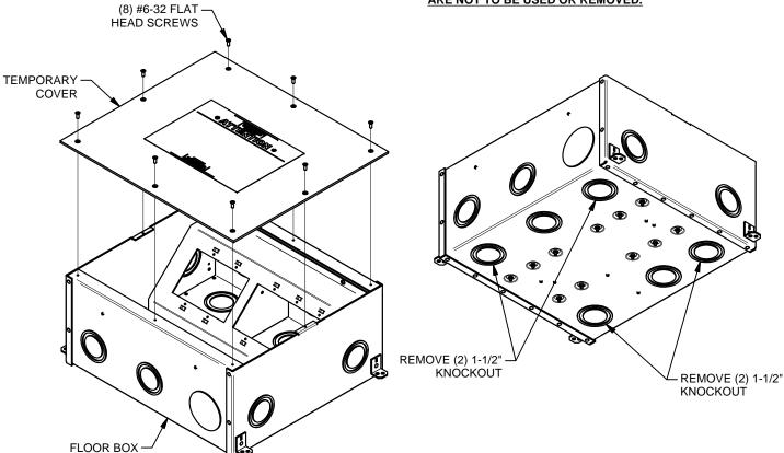
5. INSTALL INTUMESCENT-LINED FITTING AND FLOOR BOX LEVELING BOLTS AS SHOWN.
