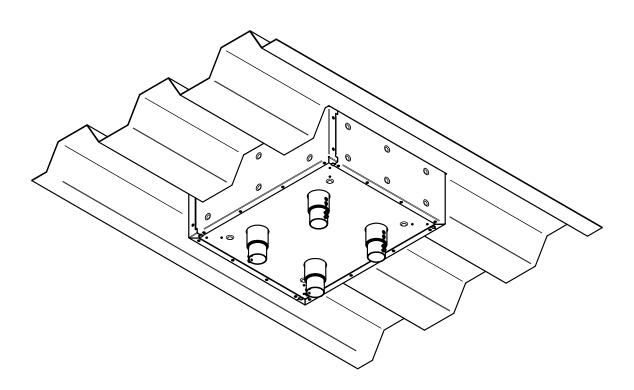
9. PULL WIRES AND CABLES TO BOX AS NECESSARY (CONFIGURING OF GANG MOUNTING BRACKETS MAY BE REQUIRED - REFER TO FLOOR BOX INSTALLATION INSTRUCTIONS). TERMINATE WIRES AND CABLES TO ELECTRONIC COMPONENTS, AND INSTALL ELECTRONIC COMPONENTS ONTO GANG MOUNTING BRACKETS. REINSTALL TEMPORARY COVER IF FINISHED COVER IS TO BE INSTALLED AT A LATER DATE.
