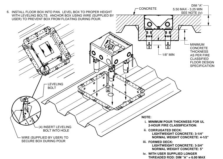
7. GANG BRACKET SCREWS AND GROUND SCREWS MUST BE IN PLACE AND BOTTOMED TO ENSURE SCREW VOIDS AFTER POUR. REINSTALL TEMPORARY COVER. FILL VOIDS BETWEEN DECK CUT-OUT HOLE AND PAN WITH TAPE OR CAULK TO PREVENT CONCRETE LEAKAGE WHILE POURING. DURING POUR, A VIBRATORY TOOL MUST BE USED TO ENSURE COMPLETE FILL OF CONCRETE SURROUNDING THE FLOOR BOX WITHIN THE PAN ASSEMBLY.
