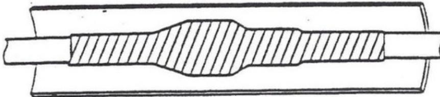
4. Tightly wrap two layers of electrical tape over and 2 inches (5.1 centimeters) beyond the mastic material.
