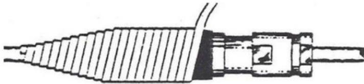
3. Tightly wrap two layers of electrical tape over and 2 inches (5.1 centimeters) beyond the connector ends.
