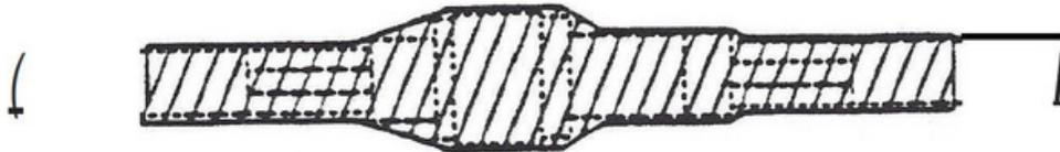
3. Wrap coax-seal weatherproofing material over the taped connectors.
