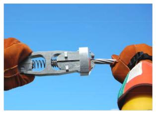
3) Fully insert wire until it reaches the stop.
