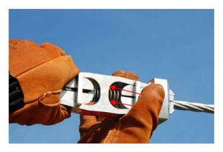
7) Jaws may be pulled back with thumb and index finger to release conductor.
