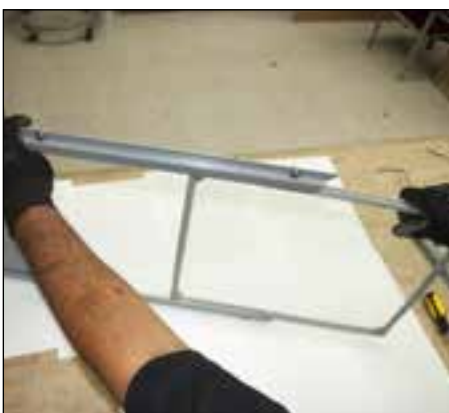
29. Slide glass lens and gasket out of lens frame and discard glass lens and gasket.
