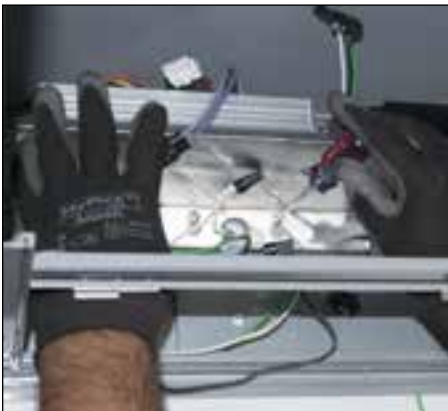
19. With provided screws, secure electronic driver tray into place.
