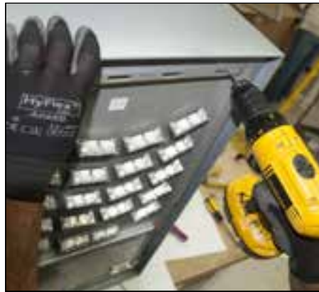
26. Secure PicoPrism deck into housing with provided screws.
