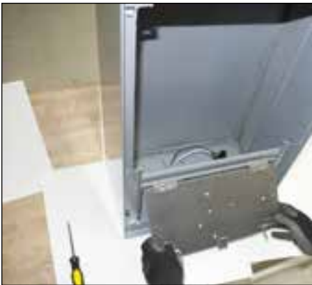
10. Slide ballast assembly door off of hinges.
