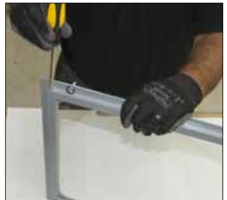
27. Remove multiple screws holding glass lens and gasket into lens frame.
