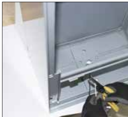
14. With wirecutters, remove harness from line voltage wires.
