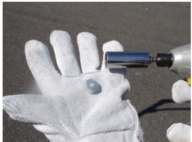
7) Use any 3/4" socket to drive the bolt until the head breaks off. Any impact, box, adjustable, speed or socket ratchet wrenches will work.
