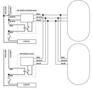
Note: One MP-Voltage Series Power Pack will supply 3 of any unit, 3 sensors, 2 sensors and 1 auxiliary or any combination.
