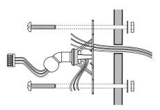
1. Insert wiring through bracket legs. Secure bracket to wall or ceiling. Refer to "Installation Options."
