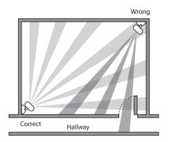
When placing the sensor in a room, do not place where the sensor is aimed out through a door. The sensor can detect hallway traffic, forcing lights-on.
