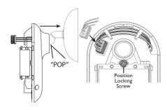
3. Snap sensor onto mounting post. Plug wiring harness into connector located on the left side opposite exit slot and place wiring under wire tabs. Align sensor and tighten adjustment screw.
