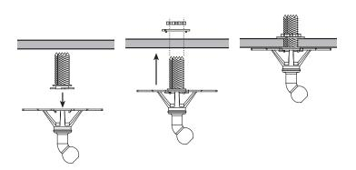
Insert ACAK into mounting bracket and twist clockwise 90° to lock into place. Screw bracket and self-cutting AKAC into ceiling tile and secure with washer and nut.
