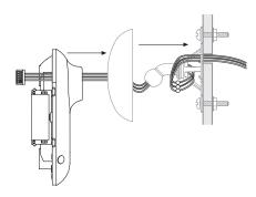
2. Connect building wiring to wiring harness with wire nuts. Snap bracket cover in place to conceal wiring and bracket. Feed wiring harness through the back of the sensor body and out exit slot.
