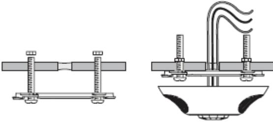
Mounting Method 1: Screw and mount twist-lock cover plate.
