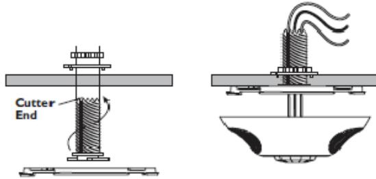
Mounting Method 2: Twist and lock threading mounting post into cover plate. Drill into ceiling tile.
