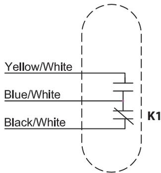
Relay Wiring For OMNI Sensor
