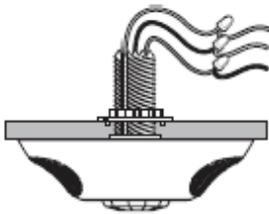
Run wiring through ceiling tile. Attach sensor body to cover plate by aligning arrows and twist locking into place. Connect wiring with wire nuts.
