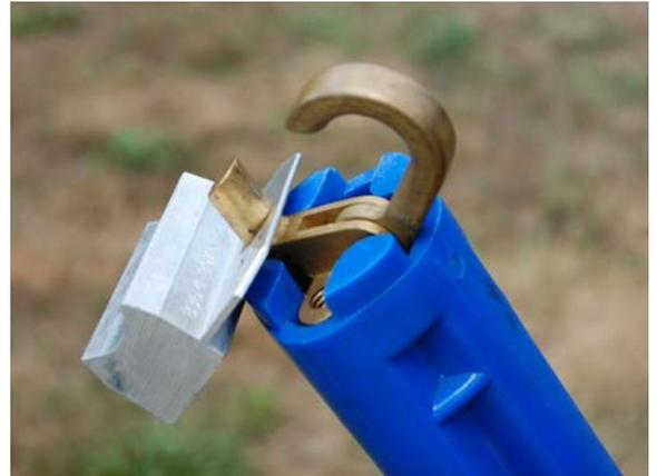
8) Insert interface on Hot-Stick in the same direction that it will be inserted into the connection. This will allow easy Hot-Stick removal.
