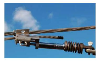
11) Use a deep socket and universal socket stick tighten drive bolt until Hex Head shears off.Make certain that socket is fully engaged.
