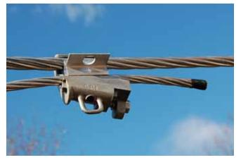
12) The bolt head should break off at 110- 130 IN LBS (12-14 NM)
