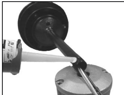
2. Install stem, coating exposed threads with thread sealant to keep moisture from entering junction box.
