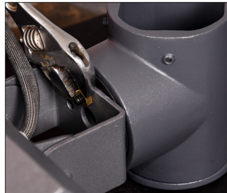
3. Torque nuts to 10 foot-pounds.
