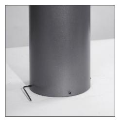
**8.** Loosen, do not remove the four (4) ¼-20 set screws at the base of the pedestal using 1/8" hex wrench.
