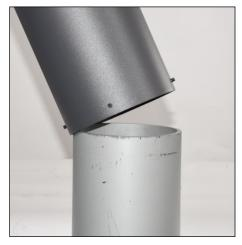
**9.** Carefully slide pedestal over Impact Post assembly and orientate as desired. Tighten the four (4) ¼-20 set screws at the base of the pedestal with an 1/8" hex wrench.
