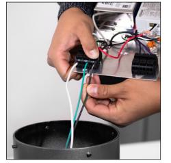
**10.** Remove head to attach incoming power supply leads to terminal block at base of driver assembly i.e black-to-voltage, white-to-neutral and green-to-ground. Also, if using DMX dimming wires, attach the terminal block with purple and grey dimming wires.
