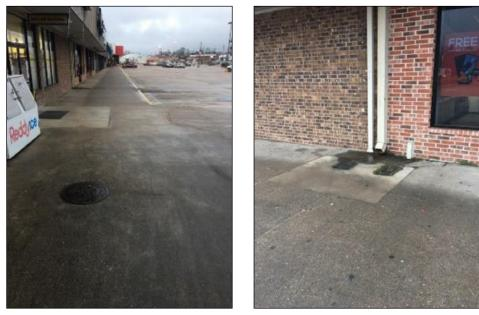
Inspect the work site for any potential conflicts that could obstruct the bollard's foundation. This includes items such as water meters, water lines, drainage pipes, electrical conduits, etc. It is advisable to use a utility locating service prior to marking any bollards.
