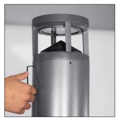
**7.** Loosen, do not remove, the four (4) ¼-20 set screws securing the luminaire head assembly to the pedestal using an 1/8" hex wrench.
