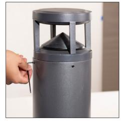
**12.** Secure luminaire head assembly in desired direction by tightening the four (4) ¼-20 set screws at the top of the pedestal using an 1/8" hex wrench.
