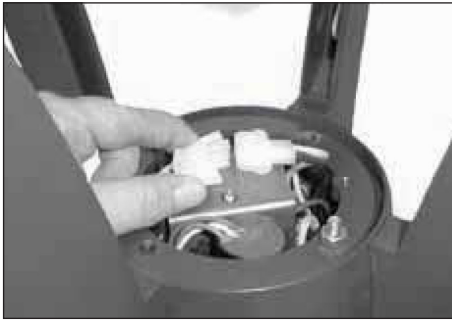
13. Disconnect wiring connectors in top of hub.
