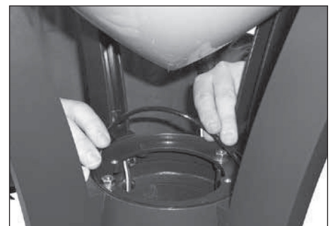
24. Install o-ring on top of retaining ring.
