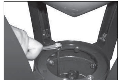
21. Re-install retaining ring and secure with (2) nuts. Tighten securely.
