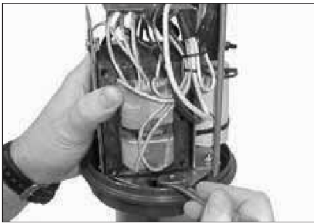
16. Disconnect pole wiring quick disconnect. Remove (2) bolts securing ballast assembly and remove.
