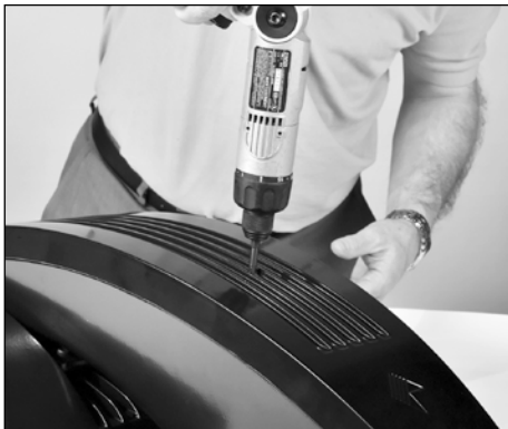
1. Loosen (2) 1/4" -20 hex socket bolts with 3/16" hex key.
