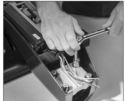
3. Loosen (4) 3/8" hex bolts with 9/16" socket and ratchet.
