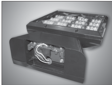
14. Speed Mount Adapter Plate for Uplight – A down luminaire can be converted to an up luminaire by removing the Speed Mount adapter Plate, rotating it 180° and reconnecting it to the back of the arm mount. The plastic connector always faces down on the Speed Mount Adapter Plate.
