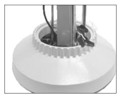
7. Connect power supply leads to the driver input leads, white-to-common, green-to-ground and blackto-voltage. Install fixture base over mounting rods.
