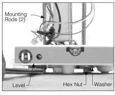
5. Level the top edge of the casting by adjusting the bottom leveling nuts using a 1/16" wrench.
