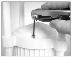
1. To install base casting to pre-set anchor bolts, base casting must be removed from fixture. Remove the 2 screws from splice compartment cover using 1/8" allen wrench.
