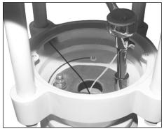
**13.** Install mounting collar over the mounting rods. Secure fixture with washer, nuts and jam nuts using %16" deep socket and ratchet.
