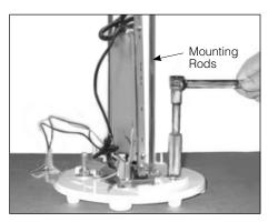
6. Tighten the upper nuts using a %16" deep socket or wrench.
