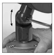
**6.** To adjust backtilt, loosen swivel screw being careful not to disengage threads. Hold fixture at desired angle and firmly tighten swivel screw.
