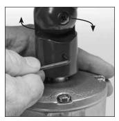
**7.** Loosen set screw to adjust fixture rotation and tighten set screw.
