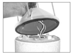
**9** Connect two 1-pin quick-disconnects. from driver assembly to quick-disconnects. on base. Align base on mounting plate bosses, insert (4) 1/4" socket cap screws and tighten using 3/16" hex wrench.
