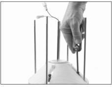
**6.** Loosen and remove (4) 1/4" socket cap screws using 3/16" hex wrench to separate base from mounting plate.
