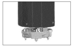
6. Place the pole body over the base casting and slowly turn until it drops into retaining slots. Then, twist clockwise 45 degrees to lock pole onto base casting.
