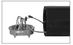
5. Pull fixture wires out from inside of riser and make connections to field wires, i.e. green-to-ground, white-tocommon and black-to-voltage.
