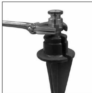
**2.** Tighten coupling onto mounting device.
